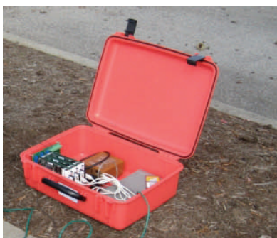
Sensor controller, location, and communication box.
